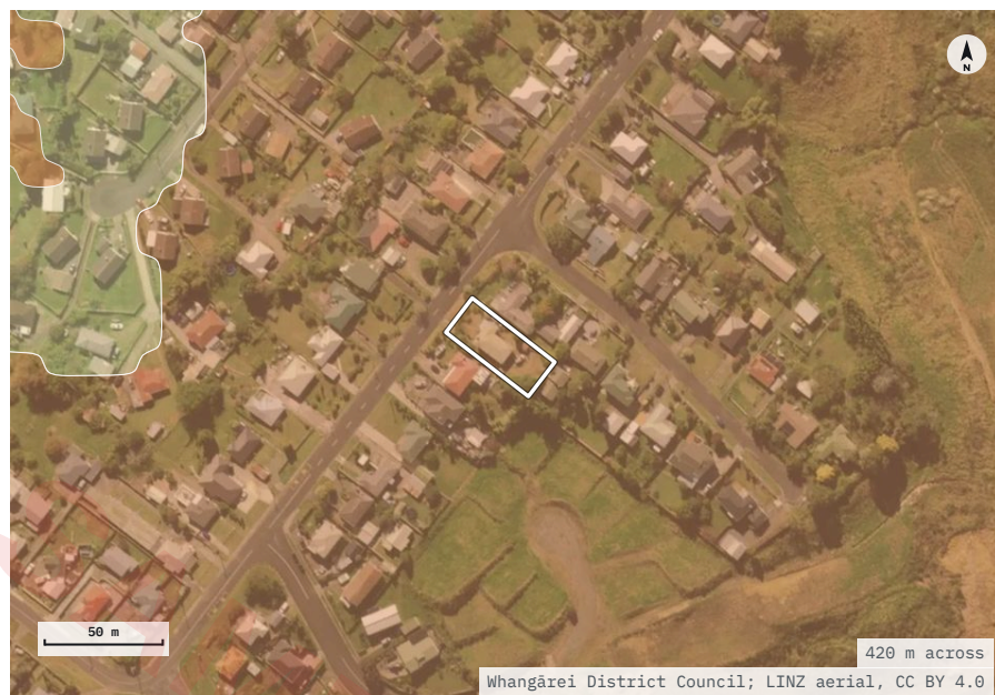
FIGURE 13. Whangārei District Council land instability mapping round the property (white). Each area is coloured by its landslide susceptibility class.
